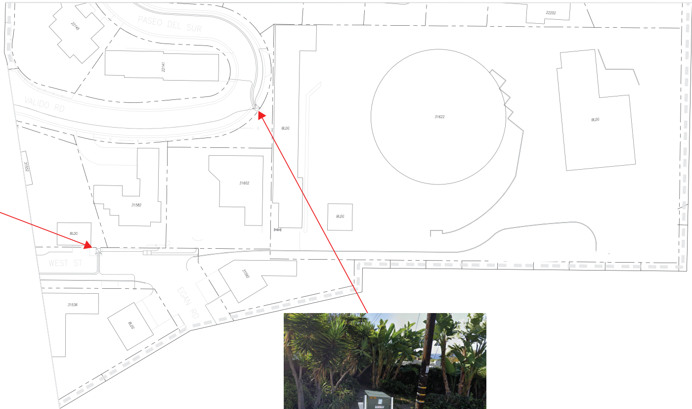
SDGE PAD-MOUNTED TRANSFORMER 36" x 33" X 26" (DARK GREEN FINISH) W/ TWO BOLLARDS
