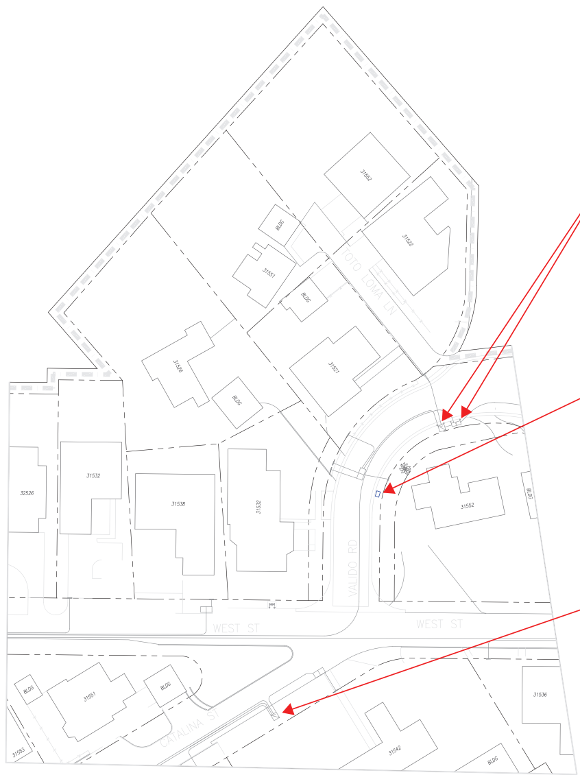
SDGE TERMINATOR CABINET 66" x 22" x 33" (DARK GREEN FINISH) W/ TWO BOLLARDS SDGE PAD-MOUNTED TRANSFORMER 36" x 33" x 26" (DARK GREEN FINISH) W/ TWO BOLLARDS
