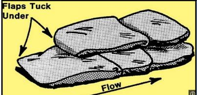
When stacking sandbags care should be taken to ensure the bags are placed parallel to the flow of water and that the stack is stable; if bags are tied flatten and flare the tied end. If bags are untied fold the open end to from a triangle and overlap them completing a layer at a time.
