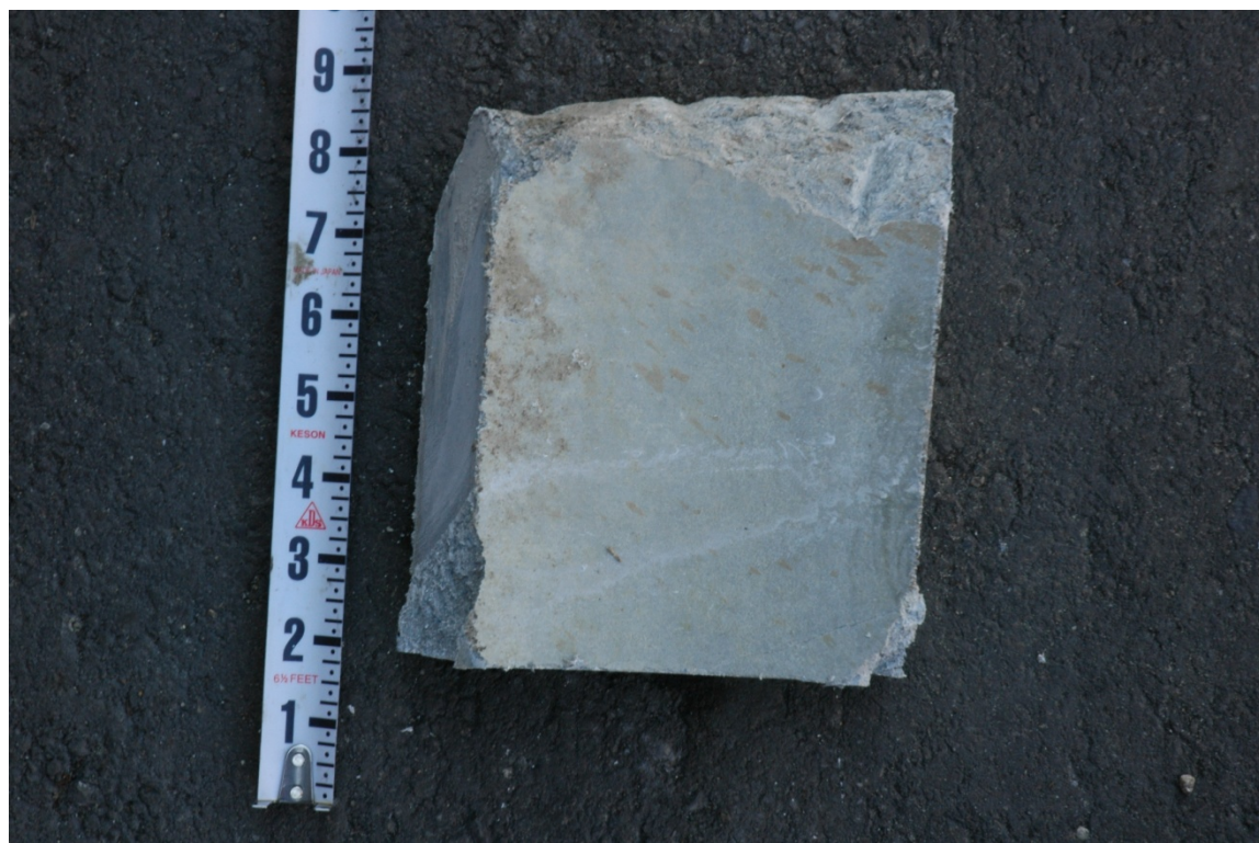
Figure 12. Petrographic sample removed from asbestos cement pipe.
