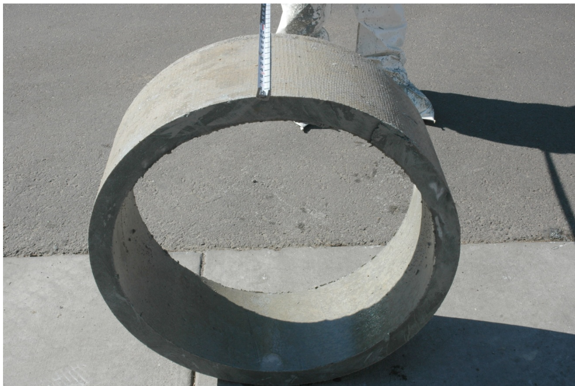
Figure 11. Ring sample removed from asbestos cement pipe.
